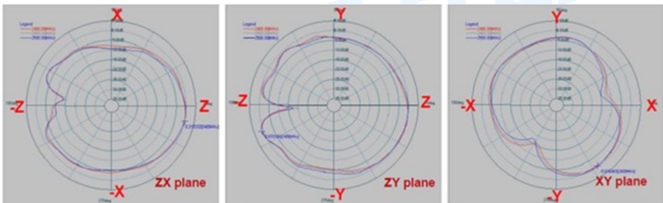
Figure 4. Antenna Radiation Pattern of USB DONGLE
