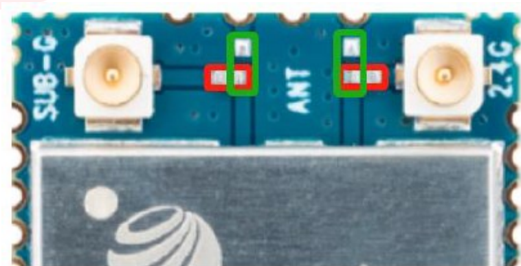
Figure 8. Antenna Output Mode Modification of RF-TI1352P2
