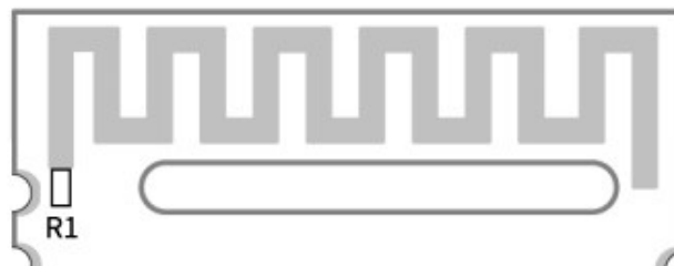
Figure 9. Antenna Output Mode Change of RF-BM-BG22A1
