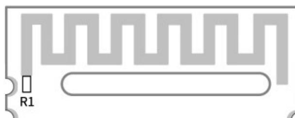
Figure 8. Antenna Output Mode Change of RF-BM-BG22A1
