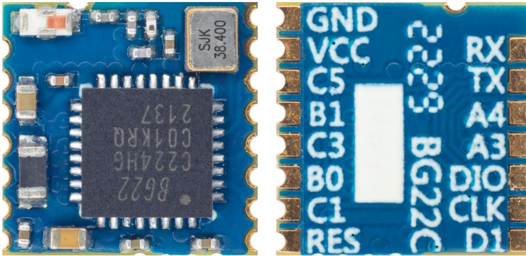
Figure 8. Module Photos of RF-BM-BG22C3
