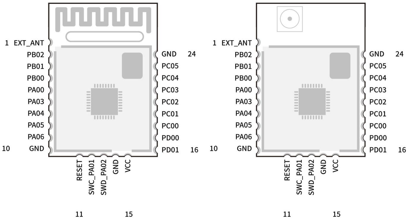
Figure 4. Pin Assignment of RF-BM-BG22Ax(I)
