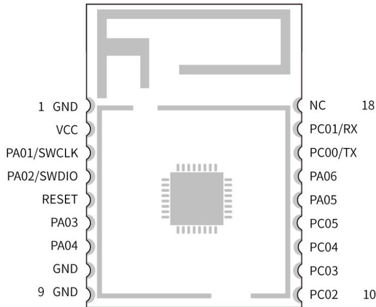
Figure 7. Pin Assignment of RF-BM-BG22B1
