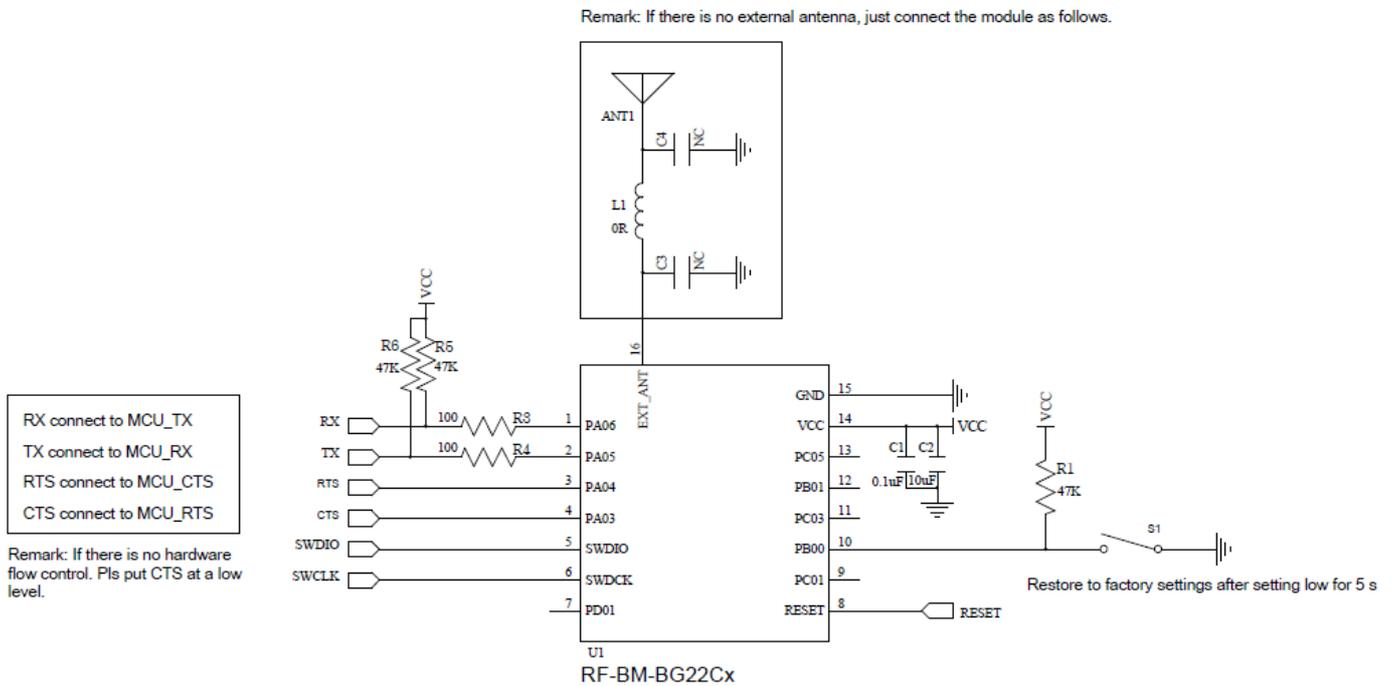
Figure 19. Reference Design of RF-BM-BG22Cx
