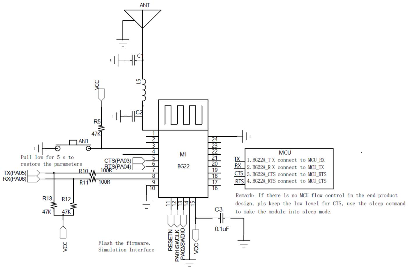
Figure 17. Reference Design of RF-BM-BG22Ax(I)
