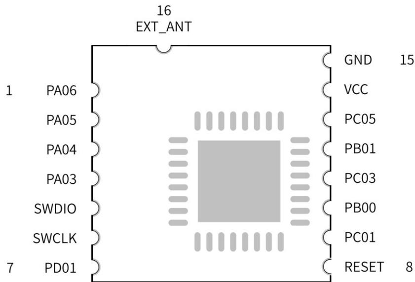
Figure 9. PCB Footprint of RF-BM-BG22C3
