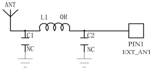
Figure 14. Reference Design of the External Antenna
