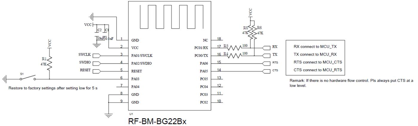
Figure 18. Reference Design of RF-BM-BG22Bx
