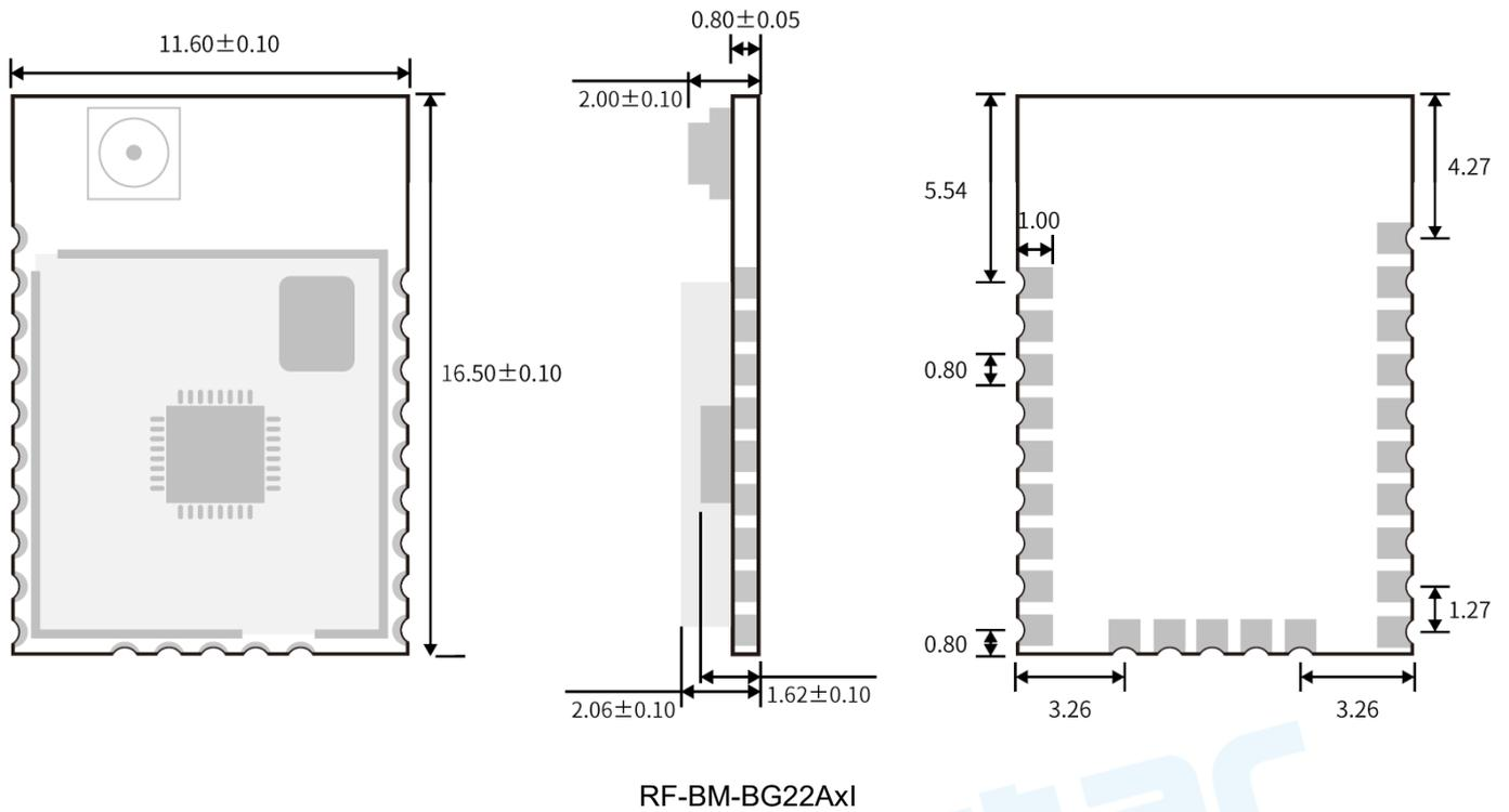
Figure 3. PCB Footprint of RF-BM-BG22Ax(I)
