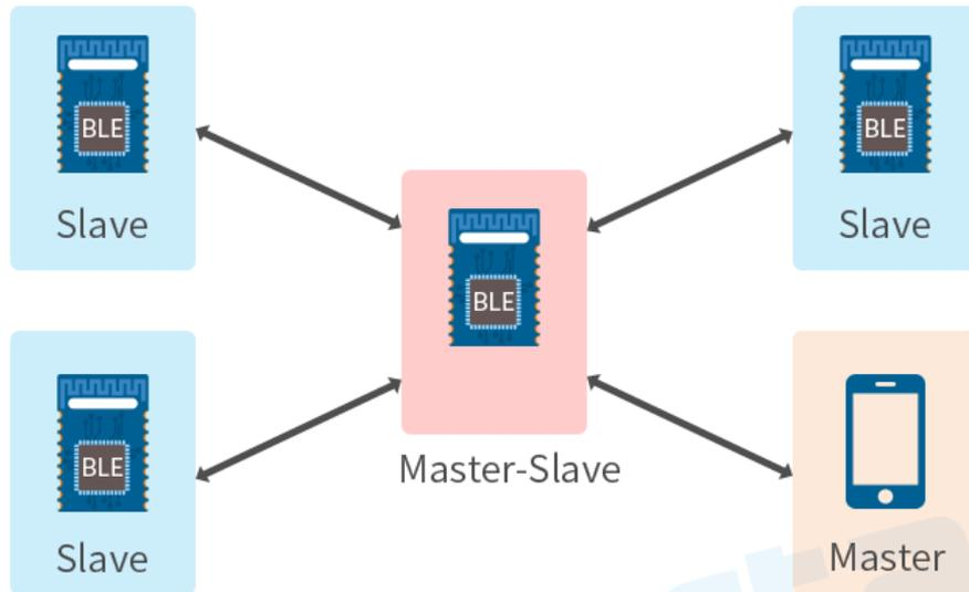
Figure 1. Multi-Connection Diagram
