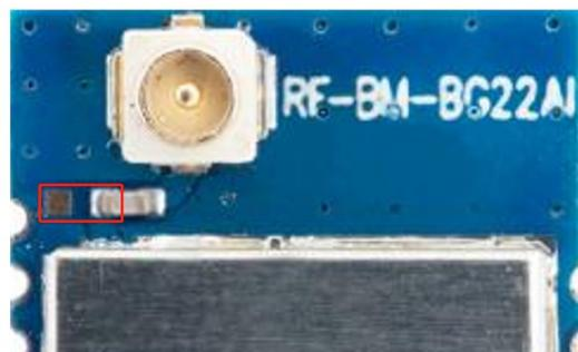
Figure 13. Antenna Output Mode Change of RF-BM-BG22A1I
