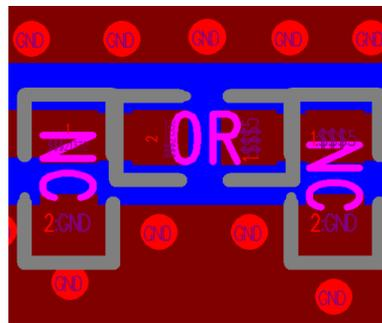
Figure 15. Reference Design of the External Antenna Traces
