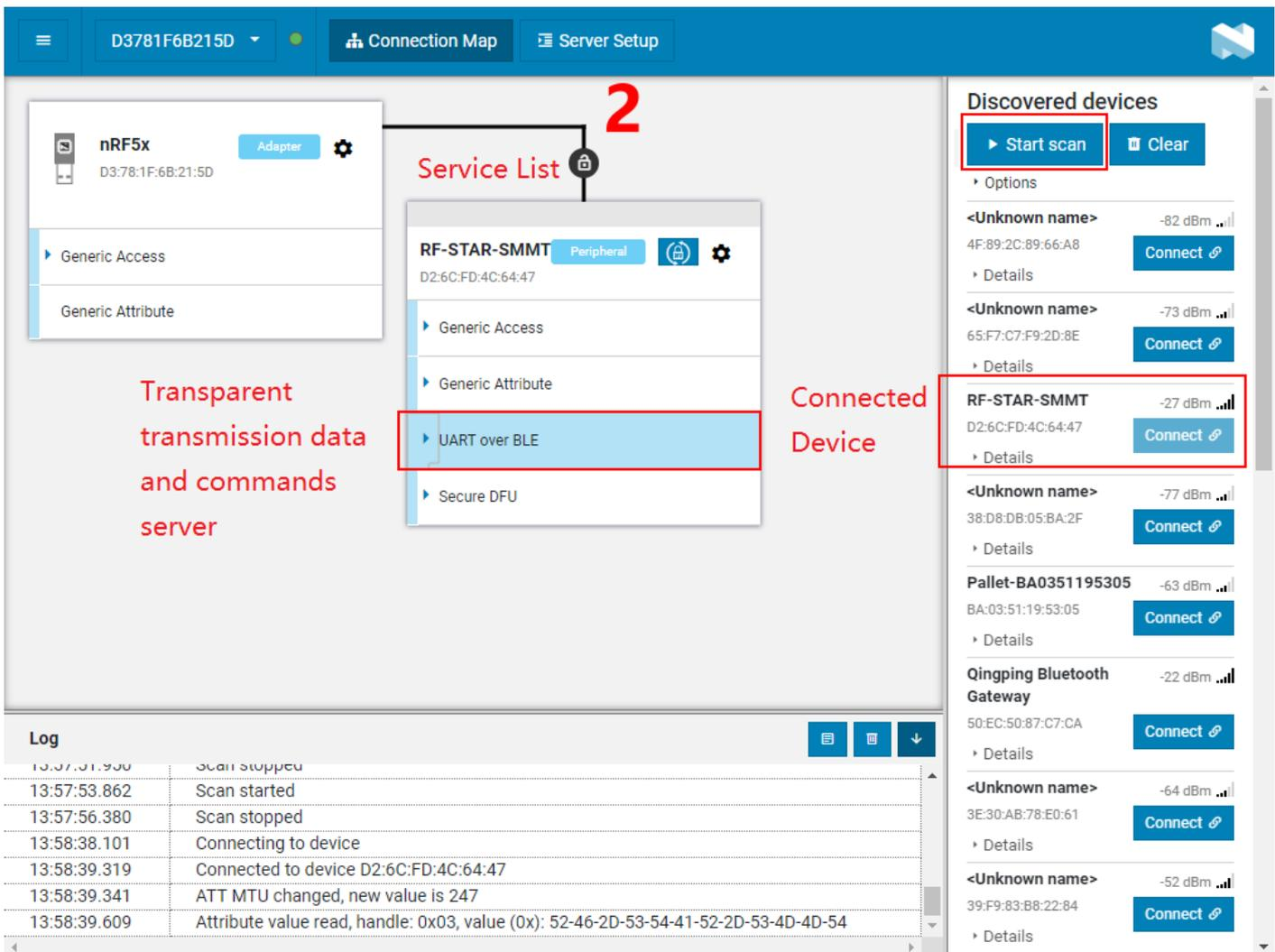
4. After the device is successfully connected, select to open the "UART over BLE" channel (as shown in the figure above), enable the Notify of the receiving channel, and then start the two-way data transparent transmission and AT between the module and the PC (with the help of Dongle as the master device) Ordered. As shown in the following pictures:
