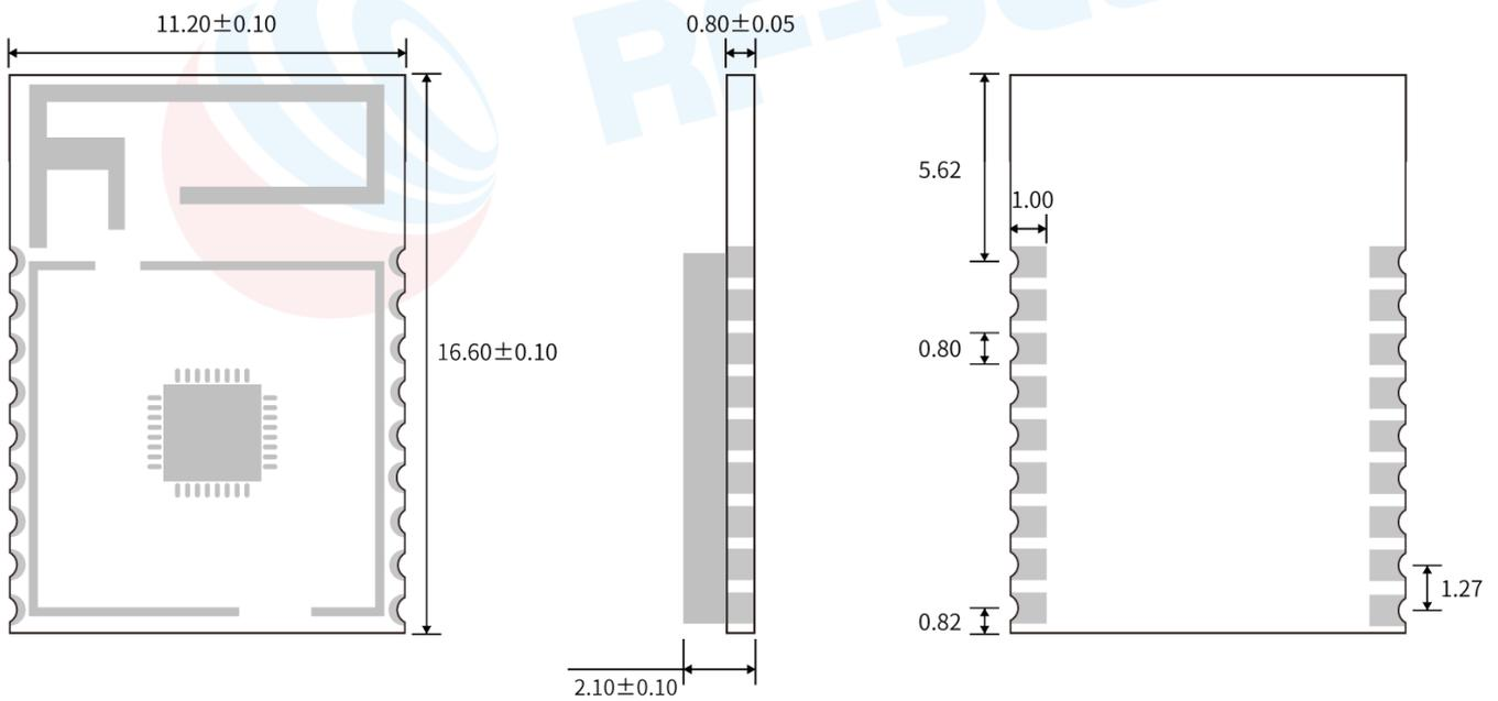
Figure 6. PCB Footprint of RF-BM-BG22B1
