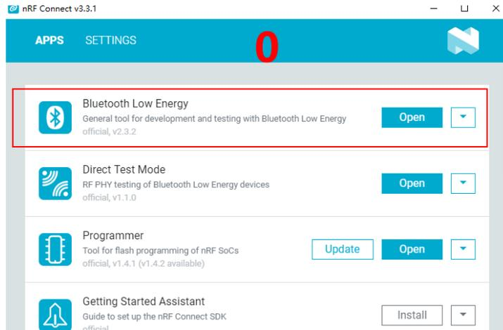
2. After installation, click the Open button and the operation interface will appear. At this time, you need to select the corresponding Dongle device for normal use. Click Select device to pop up the device name, and then click to select the corresponding device (this device name corresponds to the MAC address of the device)
